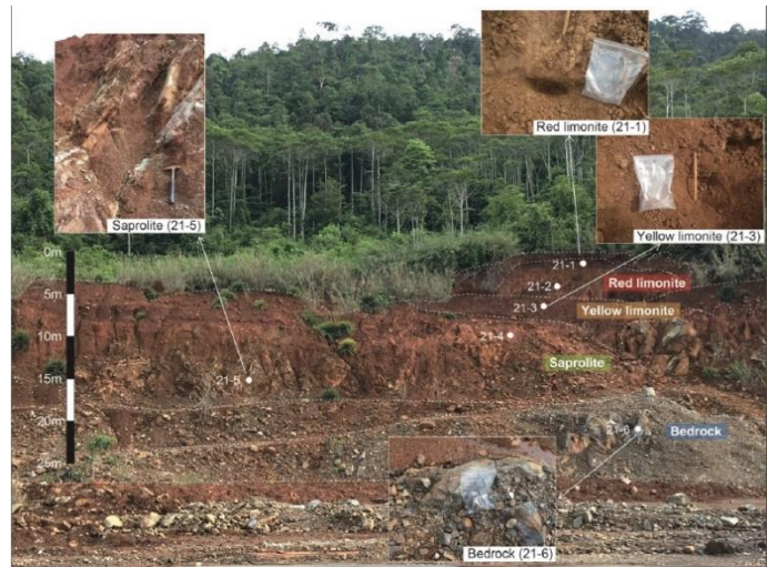
Figure 10: Cross section of nickel laterite ore vein at USSU Mine, Sulawesi
