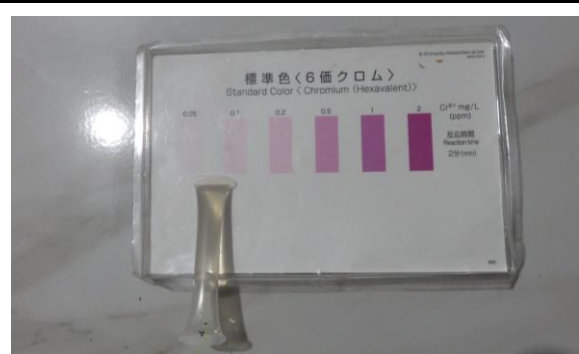
Results of simple Cr(VI) detector tube test on the community water in Asuli village (0.05 mg/L) (Photo: October 23, 2022)
